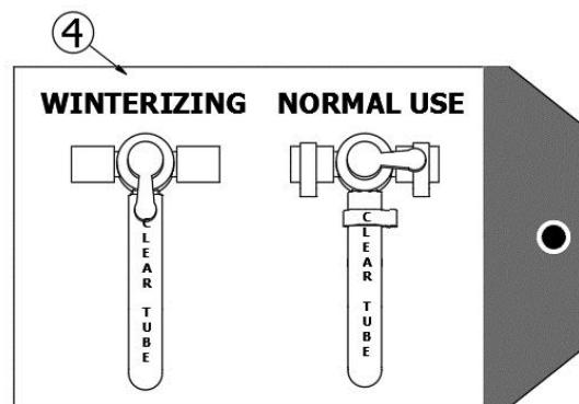
1. 601240-01      Tubing 1/2 I.D. X 3/32 Wall Thick
