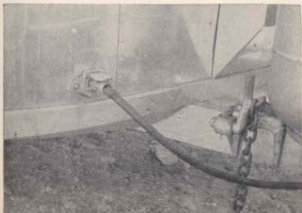
BATTERY CHARGING line between car and trailer charged the trailer 12-volt storage battery at all times.
