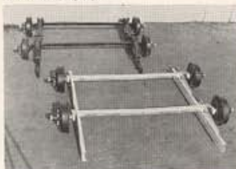
Dura-Torque axle (bottom) shows how torsion bars replace old fashioned leaf springs. Spring trouble is eliminated!
