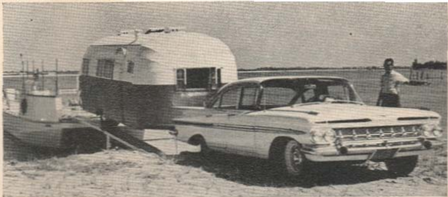
Evinrude offers complete plans for constructing this craft, which is designed to carry a conventional travel trailer as the "cabin"; catamaran hull is 40 feet.
