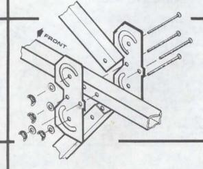
Install corner reflectors on antenna boom with brackets and hardware as shown
