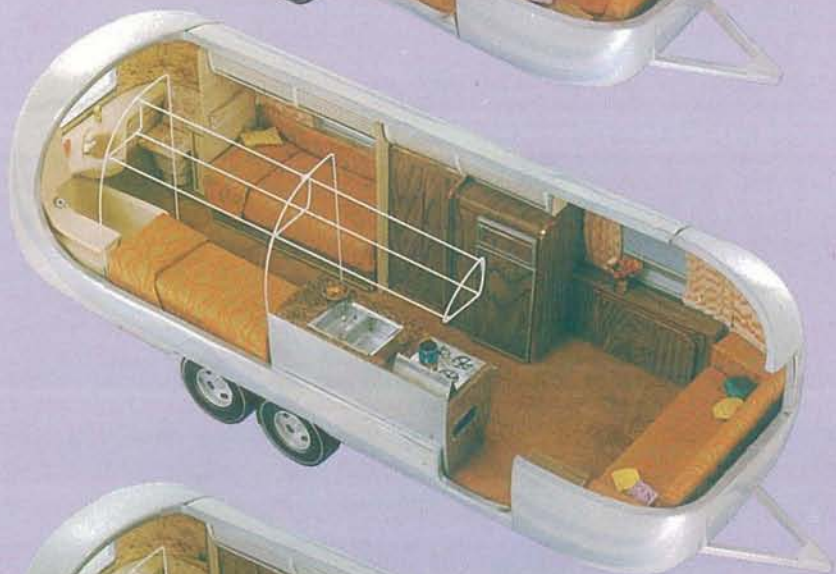
27 FT. OVERLANDER TWIN REAR BATH (International Land Yacht) Hitch Wt. 515 lbs. Total Wt. 4575 lbs.
