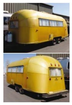
Restored trailer wheel wells have flat tops again. New gold anodizing has weathered since 1996.
