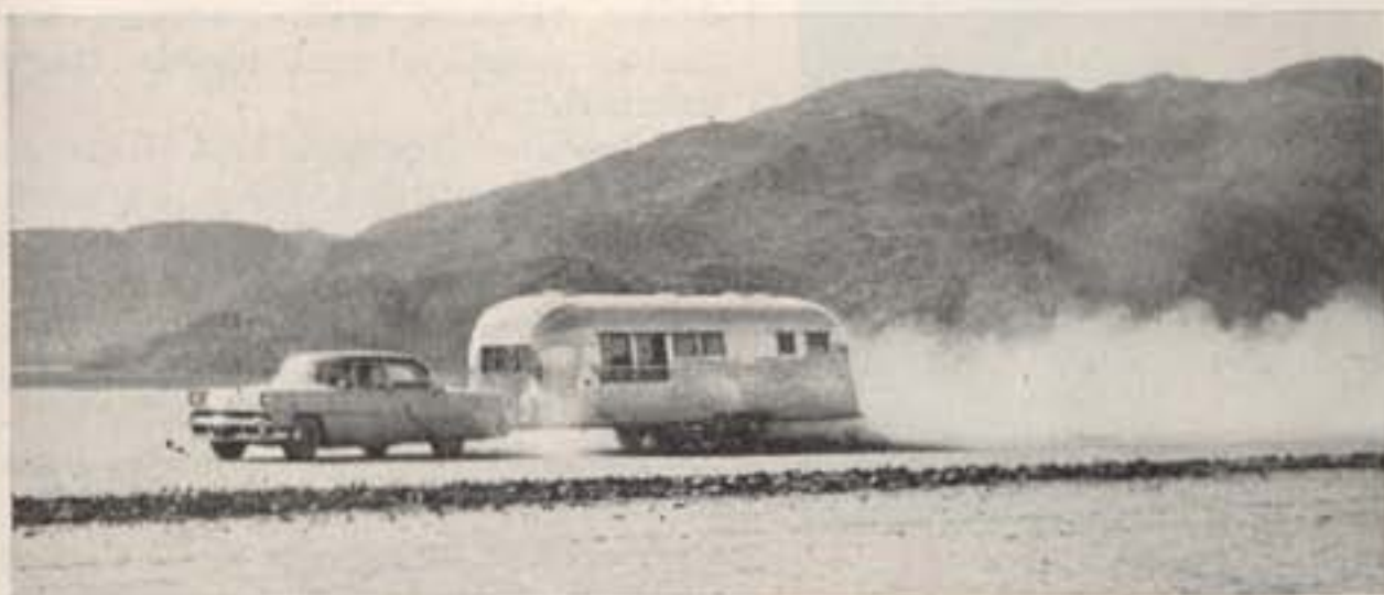
High speed runs netted 91.6 mph behind stock Mercury. Airstream all-aluminum construction means feather weight, low resistance.
