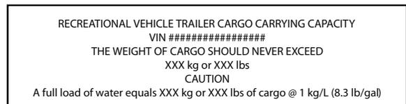
Airstream weighs the trailer as finished to arrive at the trailer's weight. That number is subtracted from the GVWR of the trailer and listed under THE WEIGHT OF CARGO SHOULD NEVER EXCEED on the tag. The total weight of any and all cargo, including dealer modifications or additions, water, and propane should never exceed the number listed.
