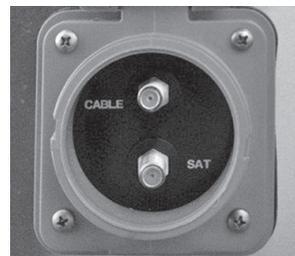
Your unit is pre-wired for a portable satellite antenna. The exterior inlet is located on the side or rear panel of the trailer and is labeled for your convenience. The interior pre-wire, consisting of a 2-pin power/ground connector and a coax cable pigtail, is located in the front roof locker under the Blu-Ray player.
