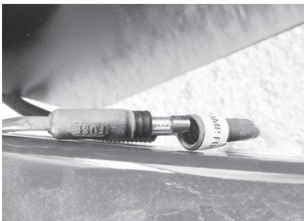
Should an electrical failure occur, first check to make sure the fuse is not blown. If the fuse is not blown place manual override handle into alignment tube and engage drive pin. Rotate handle counterclockwise to raise or clockwise to lower the camper.
