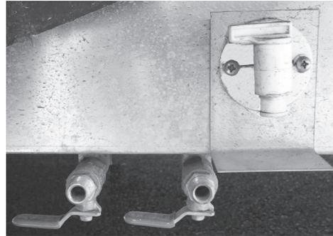
Under the trailer are galvanized steel boxes that are a few inches lower than the trailer frame. These boxes are insulated exterior tank pans and they support the freshwater and holding tanks. Petcocks open with a 1/4 turn; line drain valves are open when the widest part of the oval valve handle aligns with the water line.
