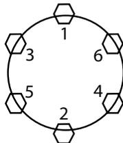
If you notice wheel wobbling, or hear a rattling sound coming from a wheel, especially at low speeds, a wheel lug nut may have come loose. This problem is usually caused by improper tightening, or by faulty or damaged lug bolt threads.
