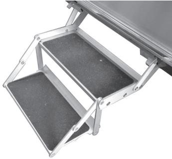
To operate the step, lift up on the front of the step and pull straight out until step locks into place. Some units will be equipped with a double step. After extending the step, the second portion folds out. To store the step, fold it back into position, lift the front slightly and push the step back into its storage area.
