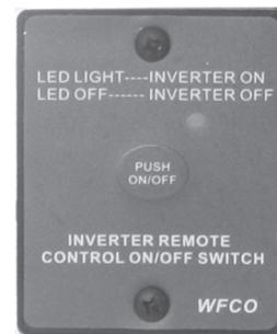
The 1,000 Watt inverter converts 12-volt electricity from your batteries into 120-volt power. The switch for the inverter is located under the monitor panel. The inverter powers the TV's and Blu-Ray player, as well as, additional labeled 120-volt receptacles.
