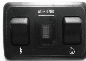
The switch used to light your electronic ignition water heater is located in the bathroom above the lavatory top. Normally, the burner will ignite in just a few seconds unless your LPG system has not been used for some time and air may have filled the lines. The system will go into safety lockout, after 3 failed ignition attempts, before the air is expelled. If this happens the red indicator light will come on. Turning the switch off for 30 seconds and then back on reinstates the ignition mode.
