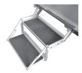
To operate the step, lift up on the front of the step and pull straight out until step locks into place. After extending step, the second portion folds out. To store the step, fold it back into position, lift the front slightly, and push the step back into its storage area.
