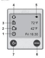
Alde's control panel is a 3.5" touch screen that makes it easy to navigate through the various functions. The control panel on the 33FB has been installed behind a removable panel between the wall and shower. On 33FB models all functions of the Alde system can be controlled from the main Firefly panel and the Alde panel will mirror the selected settings. On 30 ft. models the Alde control panel must be used.
