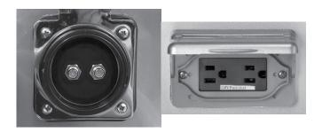
An exterior inlet for TV/Satellite and an outlet for a 120 volt receptacle is located on the side of the trailer and are labeled for your convenience.
