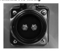
Your unit is pre-wired for a portable satellite antenna. The exterior inlet is located on the side or rear panel of the trailer and is labeled for your convenience. The interior pre-wire, consisting of a 2-pin power/ground connector and a coax cable pigtail, is located in the front roof locker under the Blu-Ray player.
