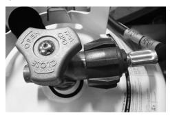
The LPG tanks are equipped with fill valve connections **RV Type I Acme**. The large, green, nylon swivel nut is a right-hand thread and is designed for hand operation only.
