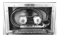
Classic units are equipped with a stainless steel exterior shower. This shower consists of a shower hose, shower head, and water valve inside of a lockable exterior door. Water is supplied by the pump or city water hookup.
