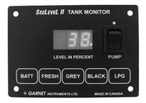
The display is the only system component that is accessed by the user. The display shown above is located inside the galley cabinet. All user input to the display is done using the five buttons along the bottom of the display.
