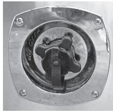
Use a tasteless, odorless, and non-toxic high-pressure hose of at least 1/2 in. diameter designed for RV use. The city water inlet is a standard garden hose thread. We suggest you carry two lengths of hose in order to reach hookups farther away than normal, plus, to have a spare.
