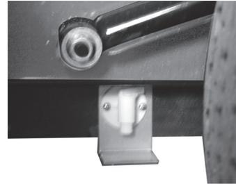
Under the trailer are galvanized steel boxes that are a few inches lower than the trailer frame. These boxes are insulated exterior tank pans and they support the freshwater and holding tanks. Petcocks open with a 1/4 turn; in-line drain valves are open when the widest part of the oval valve handle aligns with the water line.
