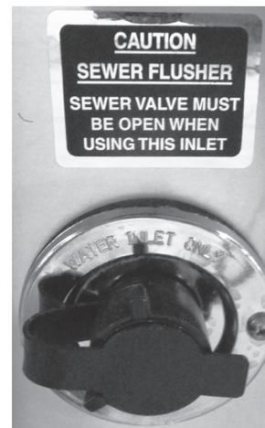
The trailer has a water hose connector specifically for flushing the Black Water Tank. To use, hook up a hose and turn on full force. Within the tank, a spray head with a multiple holed head will spray the interior surface of the tank. The vacuum breaker and check valve will be located inside the trailer above the exterior connection. In most models, this will place them under the lavatory.
