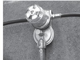
All trailers are equipped with a two stage automatic change-over gas regulator that offers the convenience of automatic changeover from empty to full gas cylinders. Both tanks are connected to this regulator.
