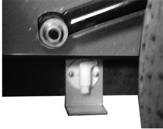
Under the trailer are galvanized steel boxes that are a few inches lower than the trailer frame. These boxes are insulated exterior tank pans and they support the freshwater and holding tanks. Petcocks open with a 1/4 turn; line drain valves are open when the widest part of the oval valve handle aligns with the water line.
