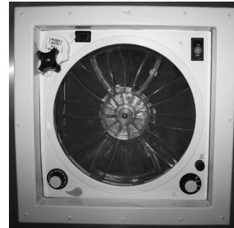
The optional high-volume roof vent system is designed to quickly exhaust stale, hot air and draw in fresh air. It is great to use when the outside temperature does not call for air conditioning, but heat has built up in your coach.
