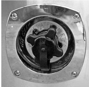
Use a tasteless, odorless, non-toxic, high-pressure hose of at least 1/2-in. diameter designed for RV use. The city water inlet is a standard garden hose thread. We suggest you carry two lengths of hose in order to reach hookups farther away than normal, as well as to have a spare.
