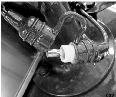
Should an electrical failure occur, remove the power head by loosening the two Allen setscrews. The jack post may now be operated manually by inserting the emergency handle into the coupling on top of the post.
