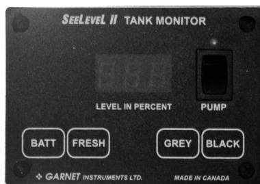
The display is the only system component that is accessed by the user. All the user input to the display is done using the five buttons along the bottom of the display.
