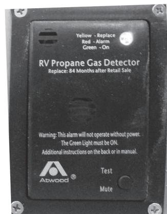
This alarm has a seven year life; see end-of-life notification in LPG detector manual. Please read the entire detector manual before operating the unit.
