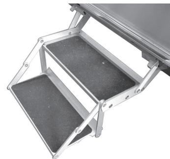
To operate the step, lift up on the front of the step and pull straight out until step locks into place. Some units will be equipped with a double step. After extending step, the second portion folds out. To store the step, fold it back into position, lift the front slightly, and push the step back into its storage area.
