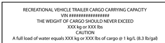
Airstream weighs the vehicle as finished to arrive at the vehicle's weight. That number is subtracted from the GVWR of the trailer and listed under THE WEIGHT OF CARGO SHOULD NEVER EXCEED on the tag. The total weight of any and all cargo, including dealer modifications or additions, water, and propane should never exceed the number listed.
