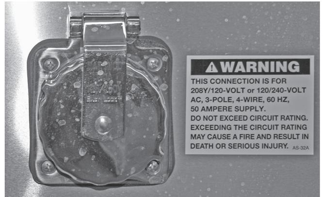
The Power Cord hookup is located on the side of the trailer. The cord may be stored in the rear exterior compartment. The power cord is plugged into the trailer receptacle and the City Power Service.
