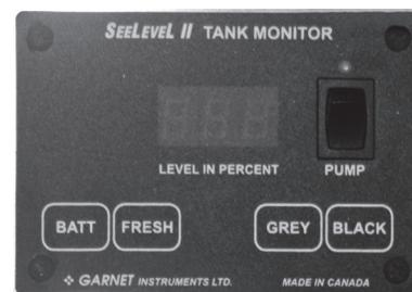
The display is the only system component that is accessed by the user. All user input to the display is done using the four buttons along the bottom of the display.
