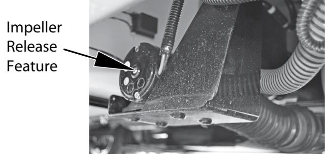
After long periods of non-use, a stuck impeller can be easily broken loose with a screwdriver inserted in the motor shaft slot. Remove the rubber boot, turn the shaft clockwise, and replace the rubber boot.
