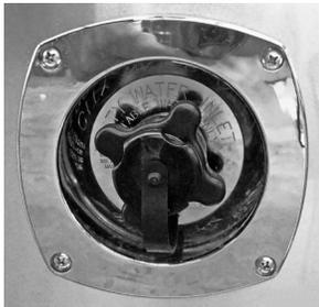
Use a tasteless, odorless, non-toxic, high-pressure hose of at least 1/2-in. diameter designed for motorhome use. The city water inlet is a standard garden hose thread. We suggest you carry two lengths of hose in order to reach hookups farther away than normal, as well as to have a spare.
