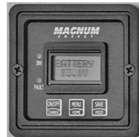
Magnum Inverter/Charger is a DC to AC inverter and a 50-amp multi-stage battery charger. It has a remote control module mounted in the roadside rear roof locker.
