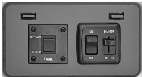
The power awning switch is located on the passenger seat pedestal. The sliding cargo door must be closed during deployment. Awning will retract, but will not extend while the vehicle is running.
