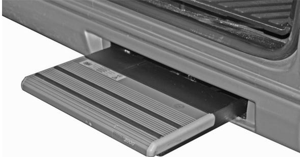
The curbside sliding door has a sliding step with auto retract, step out warning buzzer, and a lock extended switch located just inside the sliding door on the forward shower wall. Please read, understand, and instruct passengers of the following operational and safety information pertaining to the step.
