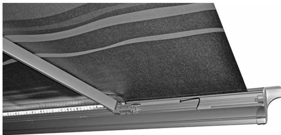
The awning will retract but won't extend while vehicle engine is running and a warning buzzer will sound.
