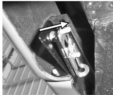
3. Pull straight down to remove cover. Once removed you can store this in one of the rear storage compartments. Reverse these instructions to reinstall.
