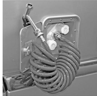
Remove and drain the hose, and open the valves before opening the low point drain lines for winterization.
