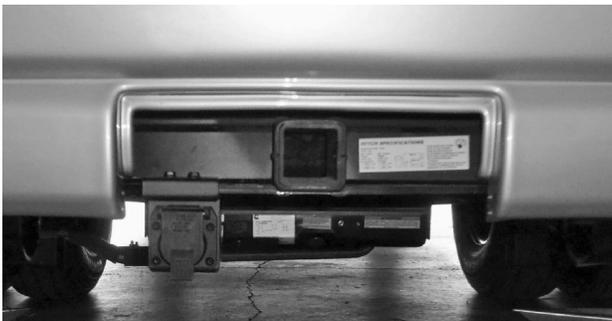
1. Kneel down behind the rear bumper. There are two side latches on the rear cover located on the lower backside of the cover. Both will need to be slid to the inside to be unlatched properly as shown below.
