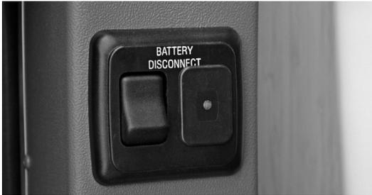
The manual disconnect switch, located inside the rear lounge door on the rear lounge model and on the front of the roadside twin bed on the twin bed model, is used to turn off power from the battery to the 12-volt distribution panel.
