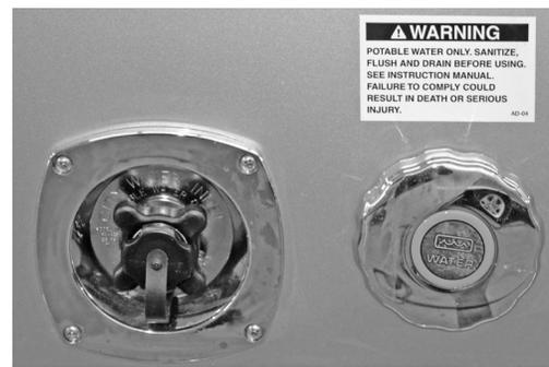
The city water inlet is a standard garden hose thread. Use a high-pressure, RV/Marine FDA-approved drinking waterhose of at least 1/2-in. diameter made from material that is tasteless, odorless, and non-toxic. We suggest you carry two lengths of hoses so you have the ability to reach hookups further away than normal. This ensures you have a spare should one fail or become damaged unexpectedly.
