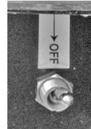
A remote switch for shutting off the gas to all appliances is located in the same compartment. The switch activates an electric solenoid which opens and closes, shutting the gas off at the tank. This switch should be turned off during the filling of the LPG tank.
