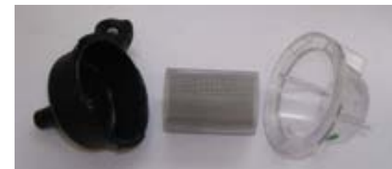
Filter on pump/ solenoid board
