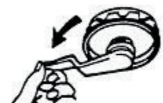
Turn elevating crank in "UP" direction until some resistance to turning is noted. Antenna is now in operating position.
