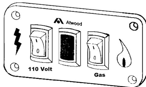
The second switch is used to operate the water heater on 110-volt power. This provides power to the heating element.
