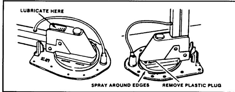
**Lubricating Rotating Gear Housing**
