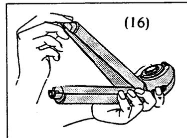
14. Reinstall filter outlet nut (21) with flat screwdriver. **DO NOT OVER TIGHTEN!**
