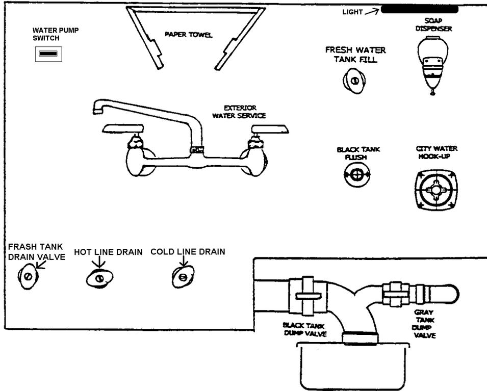
Use a high-pressure hose of at least 1/2" diameter. It should be one that is tasteless, odorless and non-toxic designed for RV use. The city water inlet is a standard garden hose thread. We suggest you carry two lengths of hose. This way you have the ability to reach hookups further away than normal, plus you have a spare hose should one fail or become damaged unexpectedly. Turn the water heater bypass to the normal flow position as described under self-contained.
