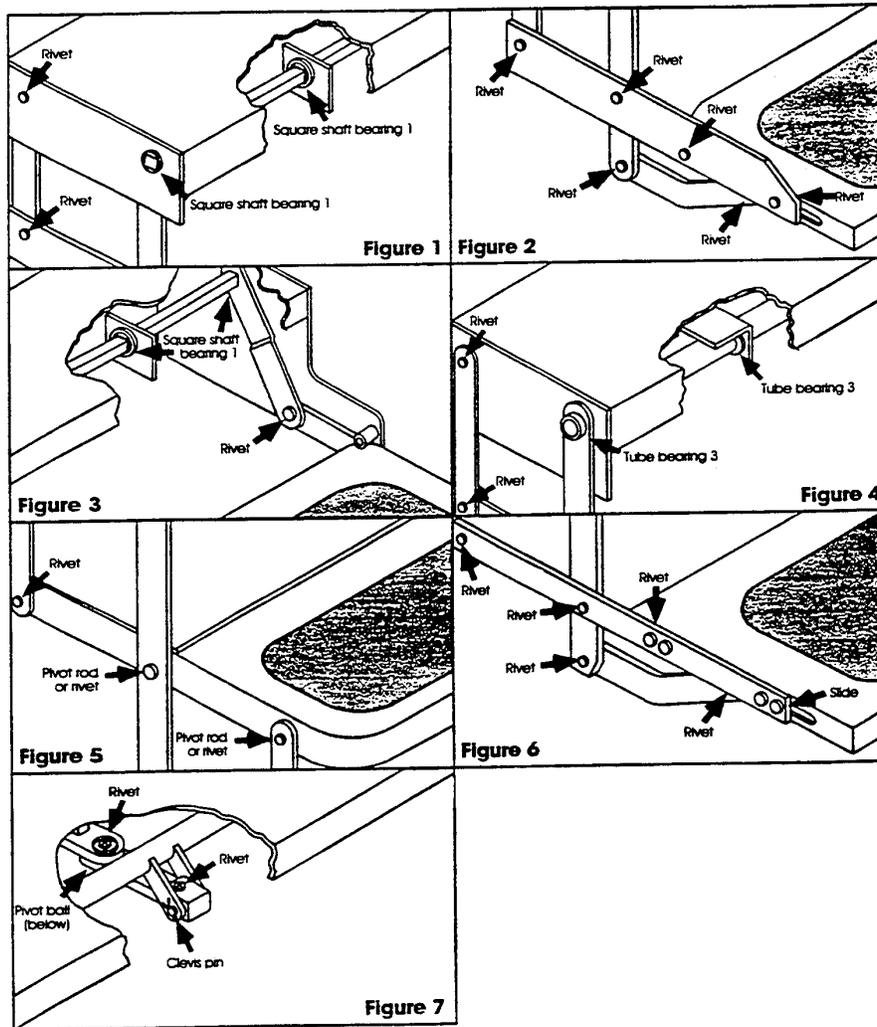
Clean all mud, salt, and road grime from step before lubricating. Lubricate all moving parts (bearings, pivot points, slides, clevis pin, and drive linkage ball) every 30 days with a good quality moisture and heat resistant penetrating grease. Kwik-Lube Spray Grease is specially formulated to lubricate Kwikie Electric Steps and is recommended for lubricating all moving parts. Refer to the figures below for lubrication locations.
