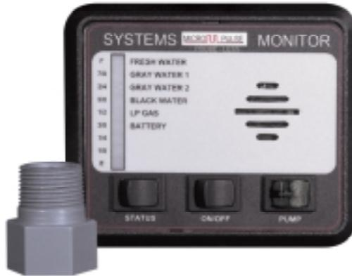
The MicroPulse System makes use of a single solid-state sensor per tank. The MicroPulse sensor measures the static (head) pressure at the bottom of the tank and transmits this information to the MicroPulse System Monitor. Knowing this pressure value, after a one-time calibration has been performed, the MicroPulse System will calculate and accurately display the tank level in 1/8 increment.
