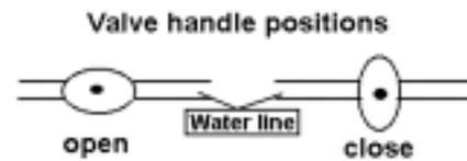
\*To by-pass the water heater for winterizing, close valves A and C and open valve B C, (See illustration).
