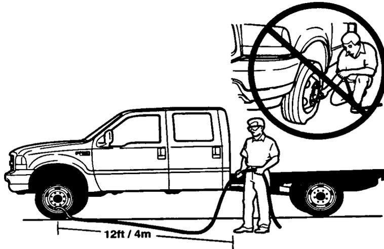
**! WARNING:** An inflated tire and rim can be very dangerous if improperly used, service or maintained. To avoid serious injury, never attempt to re-inflate a tire which has been run flat or seriously under inflated without first removing a tire from the wheel assembly for inspection. Do not attempt to add air to tires or replace tires or wheels without first taking precautions to protect persons and property.
