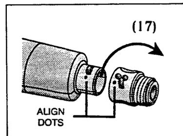
17. Reattach quarter turn connector (18) to pullout spout (19) aligning the dots on the quarter turn connector and the spout. Push the quarter turn connector onto the spout assembly and turn it clockwise, locking it in place. Return spout to the receptor.
