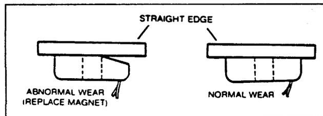
Even if wear is normal as indicated by your straightedge the magnets should be replaced if any part of the magnet coil has become visible through the friction material facing of the magnet. It is also recommended that the drum armature surface be re-faced when replacing magnets. (See Brake Drum Section) Magnets should also be replaced in pairs (both sides of an axle). Use only genuine Dexter replacement parts when replacing your magnets.
