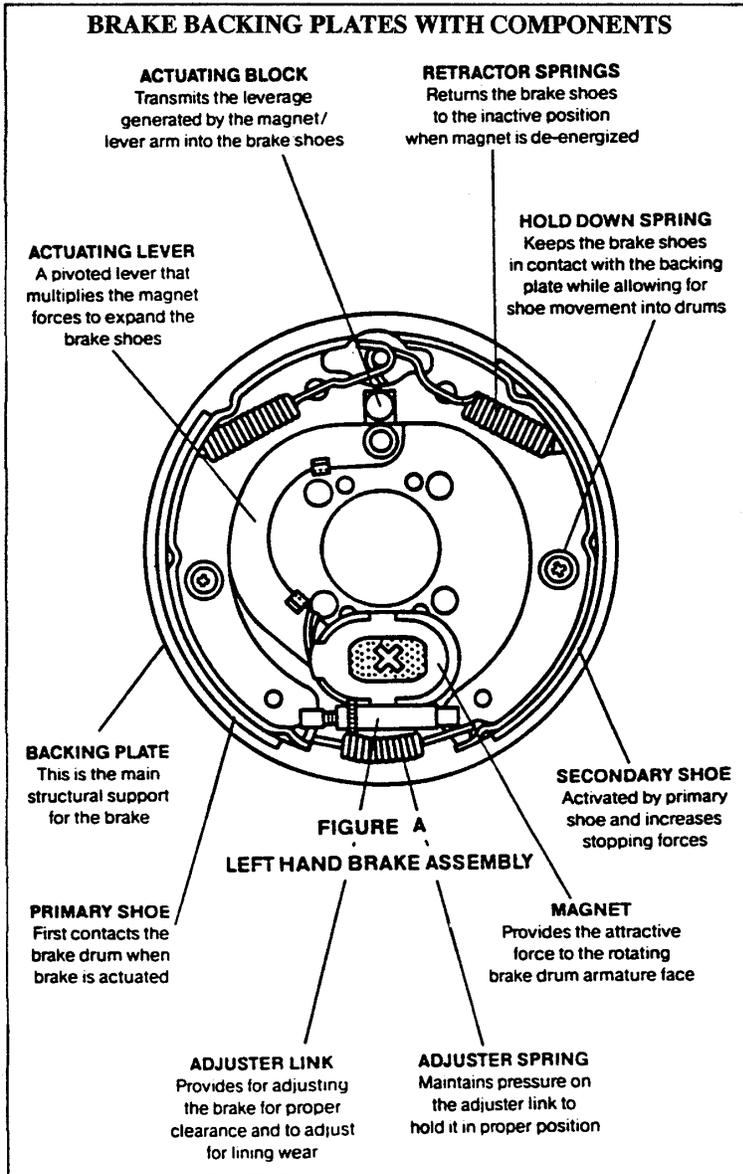
Increasing the current flow to the electromagnet causes the magnet to grip the armature surface of the brake drum more firmly. This results in increasing the pressure against the shoes and brake drums until the desired stop is accomplished.
