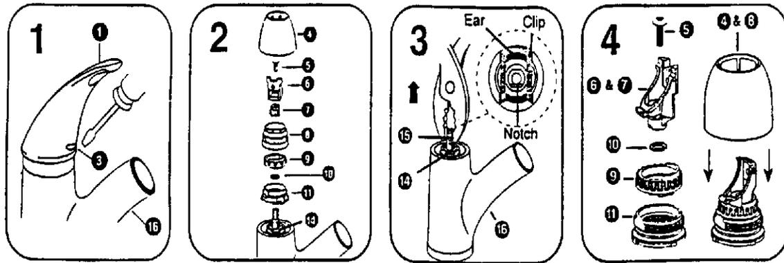
**CAUTION:** Always turn water OFF before removing existing faucet or disassembling the valve. Open faucet handle to relieve water pressure and ensure that complete water shut-off has been accomplished.
