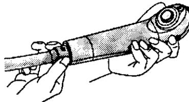
2. Disconnect the quarter turn, connector (18) from pullout spout by turning it counterclockwise one-quarter turn. Quarter turn connector will remain on the hose.
