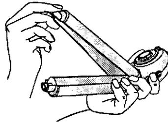
6. Reinstall the filter cover by positioning the alignment tab with the corresponding notch in the main pullout spout body and gently pushing in and down.
