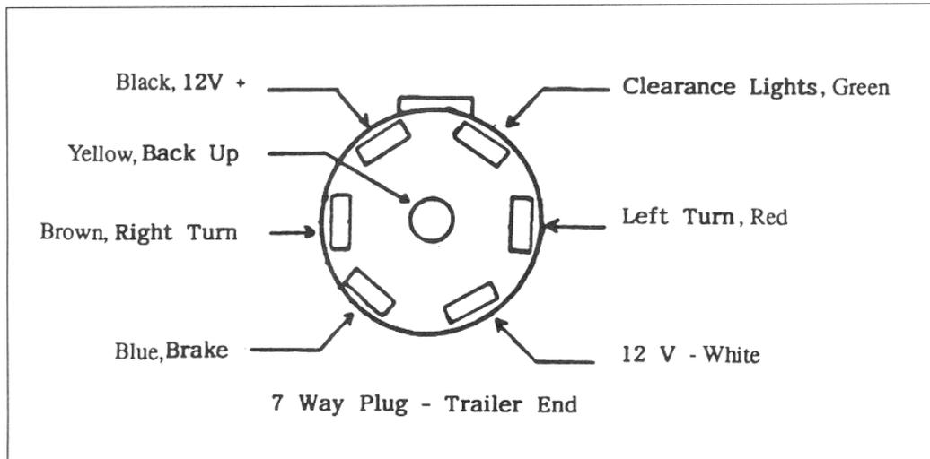
**Note:** The 7 way wire is spliced to the main harness in the area of the 12-volt distribution panel in front of the trailer.
