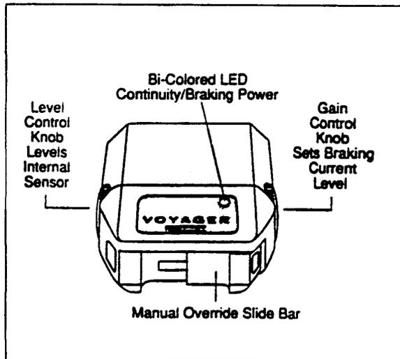
ELECTRONIC CONTROLLERS are inertially activated. The controller senses deceleration and generates an output, which reflects the inertia sensed. When your stationary, the controller does not apply the brakes unless the manual slide bar is activated.
