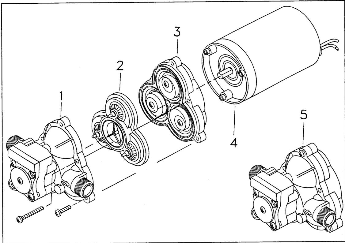
1. Switch/check valve and upper housing kit (replaces all previous switch designs)
