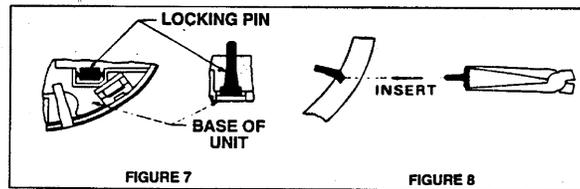
3. Using long-nose pliers grab the head of the locking pin and insert into hole located on the side of the smoke alarm. See Figure 8.
