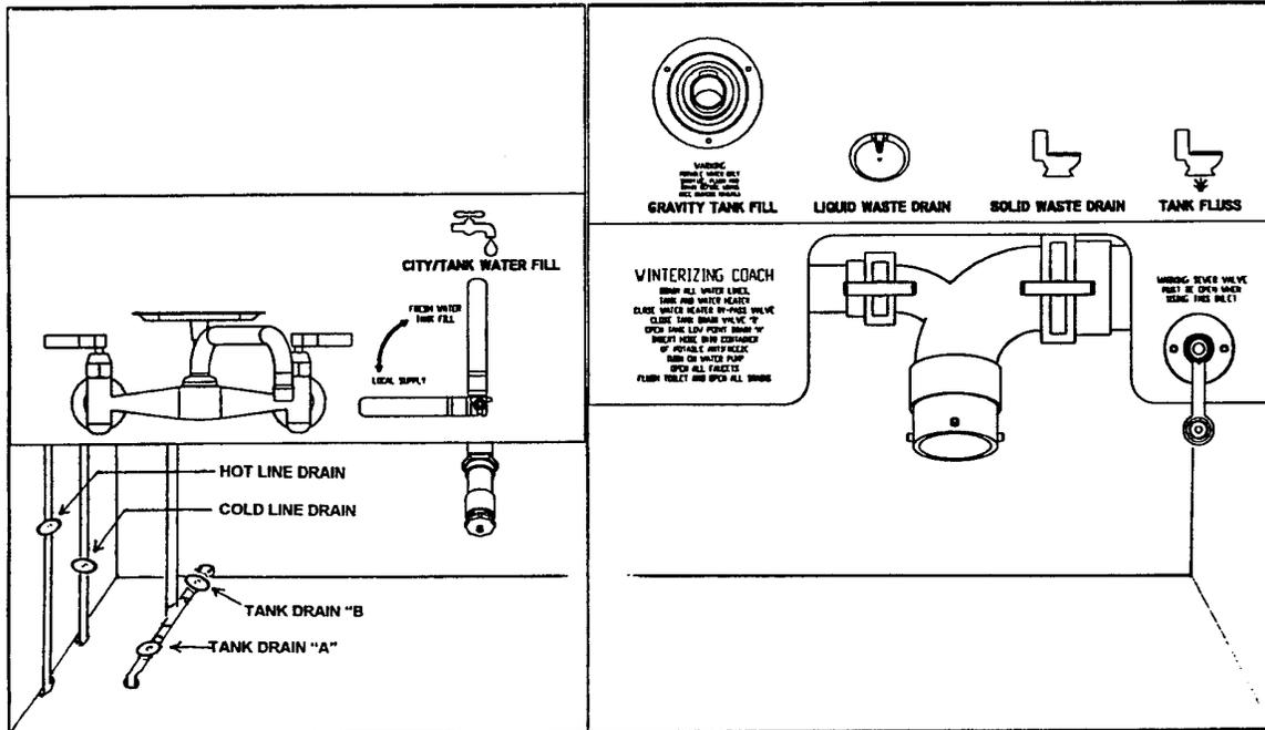
Use a high-pressure hose of at least 1/2" diameter. It should be one that is tasteless, odorless and non-toxic designed for RV use. The city water inlet is a standard garden hose thread. We suggest you carry two lengths of hose. This way you have the ability to reach hookups further away than normal, plus you have a spare hose should one fail or become damaged unexpectedly. Turn the water heater bypass to the normal flow position as described under self-contained.
