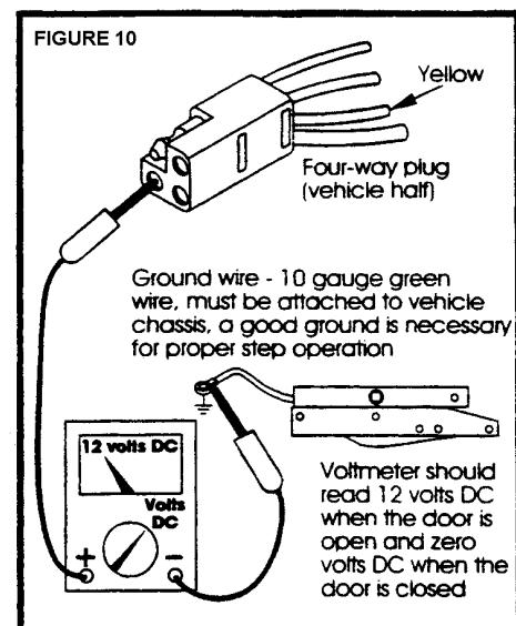
If the reading is zero when the ignition is on, check the terminal connections in the vehicle's fuse/circuit breaker and the condition of the circuit's wiring and terminal connections. **NOTE -The step wiring circuit must be independent. No other device (i.e. alarm systems, step well lights, etc.) can be connected to the step wiring circuit. Any device connected to the steps wiring can cause the step to malfunction and will void the warranty.**
