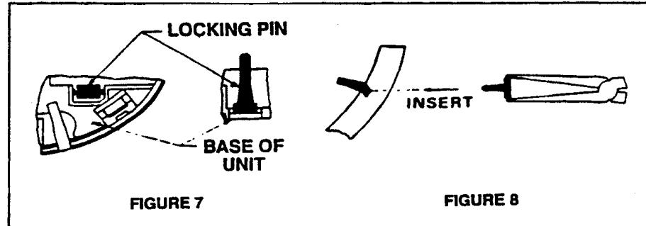
1. Remove the break-away locking pin from the unit by rocking pin back and forth.
