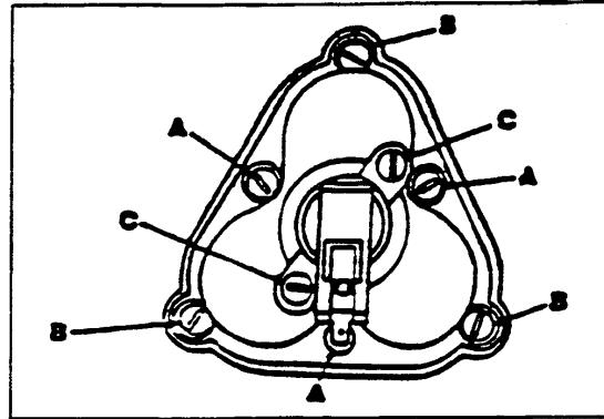
To replace a diaphragm follow the procedure used in removing the pistons. After removing the three pistons the diaphragm is loose and easily removed.
