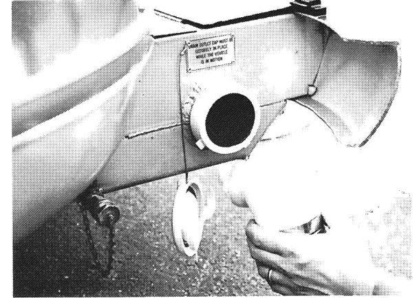
Waste Drain Hose Hook-Up
