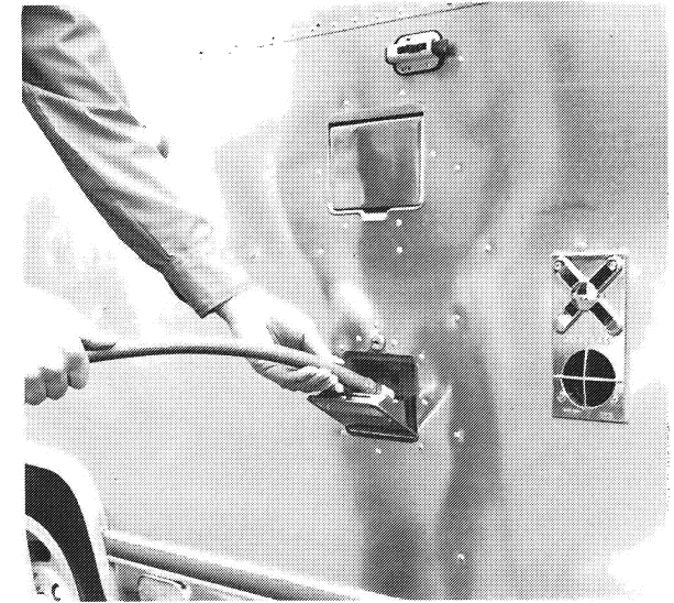
Water Tank Fill Spout
