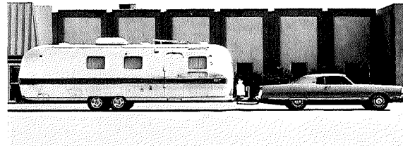
Hitch Installation Proper – Hitch ball slightly higher.
