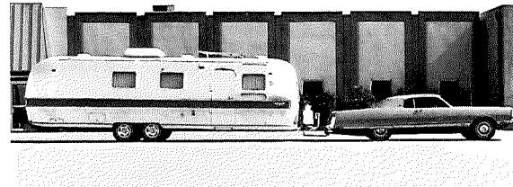
Hitch Low – Load on front wheels too light. Need more tension on load equalizing bars.
